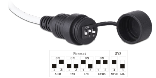
DIP Switch for Output Selection
