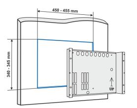
The mounting hole in the drywall must be a little greater than the dimensions of the metal base.
