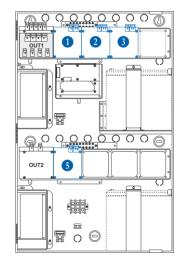
The iRIS8 will recognise 4 loop expanders -3 connected to OUT1 (numbers from 1 to 3) and 1 connected to OUT2 (number 5).
