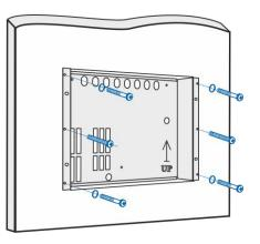
4 pcs - Screw M4x40, DIN7985 4 pcs - Washer M4 DIN 522, ø12mm
