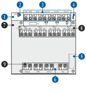
Monitored Outputs PCB. The PCB is under the Relays PCB. The elements are indicated with blue numbers.
