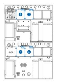
The iRIS8 will recognise 4 loop expanders -2 connected to OUT1 (numbers 1 and 2) and 2 connected to OUT2 (numbers 5 and 6). The loops will be set with the factory addresses:
