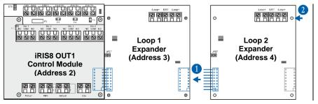
Connect the interface connectors of the first and the second loop expanders.
