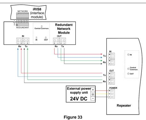
The maximum cable length between two network modules and/ or repeater panel is 1000m.
