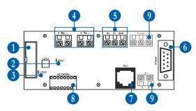
\*Note to positions 4 and 5: The using of communication protocol is enabled from the installer programming menus at level 3: System-Programming-Panel-FAT/FBF&ESPA444. You can program operation with only one of the communication protocols, respectively you can use only one interface connection. 1 – Interface ribbon cable connected to Main control module PCB (factory mounted).
