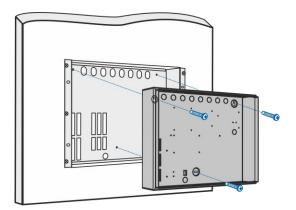
Use 3 pcs of screws M4x12 (DIN 966) for fixing the metal box of iRIS8 S to the metal base.
