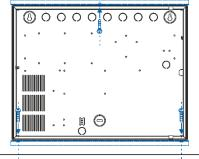
Use 3 pcs of screws M4x12 (DIN 966) for fixing the metal frame to the iRIS8 S box bottom.
