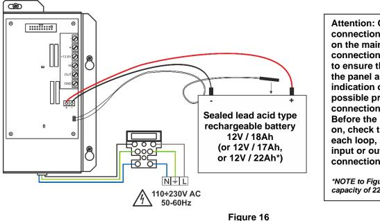
Attention: Check the earth connection cable before switching on the mains power supply – the connection must be tight and stable to ensure the correct operation of the panel and accurate LED indication on main power source for possible problems with earth connection of the panel. Before the mains supply is switched on, check the correct connection of each loop, sounder or any other input or output, and the earth connection cable.
