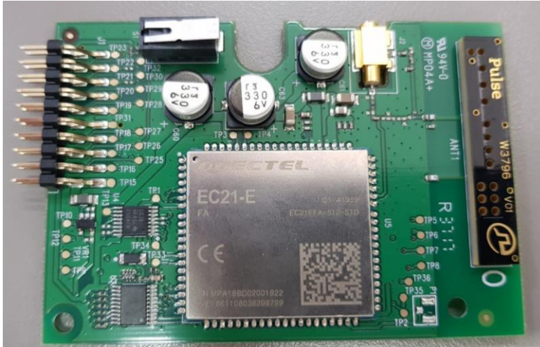
Photograph 5.1.8, 5.1.9– GPRS Module view
