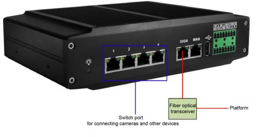
Figure 4-7 Single segment networking method
