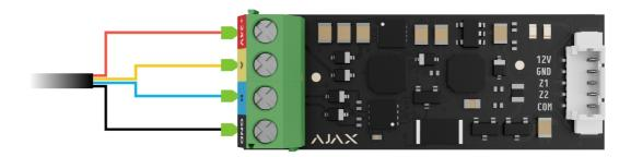
1. If Transmitter Fibra is not the last device on the Fibra line, prepare a second cable in advance. Connect the wires to the Transmitter Fibra terminals according to the figure below.
