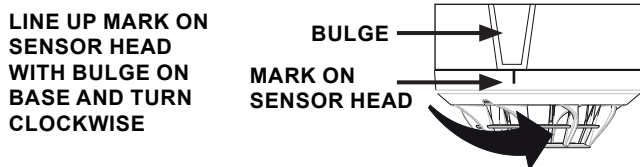
Figure 2: Attaching Sensor Head to Base
